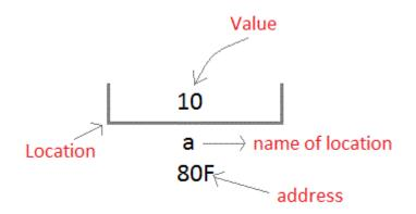
We can access the value 10 by either using the variable name a or the address 80F. Since the memory addresses are simply numbers they can be assigned to some other variable. The variable that holds memory address are called pointer variables. A pointer variable is therefore nothing but a variable that contains an address, which is a location of another variable. Value of pointer variable will be stored in another memory location.
